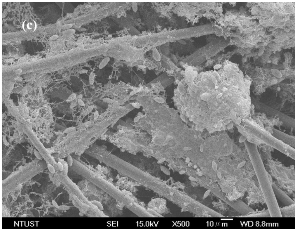
Figure 3.10. Surface Morphology of (a) Graphite felt electrode without biofilm, (b) Mixed consortia of bacterial biofilm layer encircling the graphite felt fibre electrode (c) Magnified image of the biofilm on the electrode, (d) Magnified image of the conductive pili used by the bacterial consortium as mode for electron transfer on the graphite felt surface.
