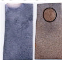
Figure 5. Fe(III) complex coated on a filter paper before (left) and after (right) exposing to amine vapor
