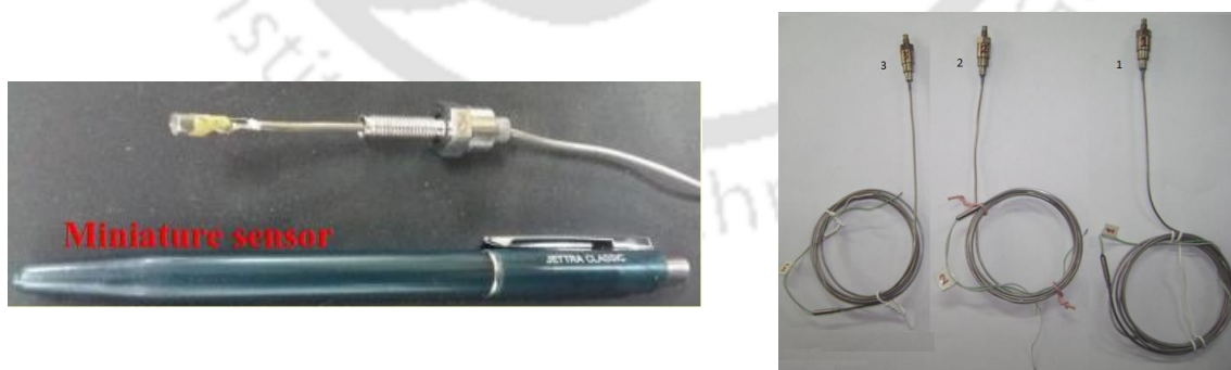
Fig. 15: (a) Miniature CSJT probe housed in a barrel, (b) packaged sensors for gas turbine engine testing
