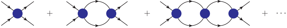
FIGURE 3.2: The bubble chain sequence of Feynman diagrams representing contributions to the S-wave B - B scattering process in the CM frame of the loop diagram arising from the local operator. The solid lines denote B-field propagators and the dark blobs denote the sum of tree-order local interaction vertices to any arbitrary order.
