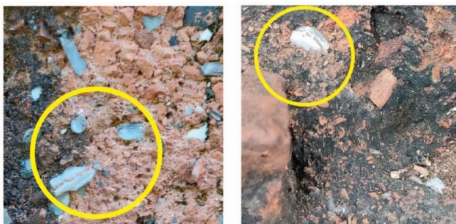
Fig. 6. 2 Zoomed in photo displaying particles of snail shells: Ghanasyam Mortar (left), Namath Kali Mortar (Right)
