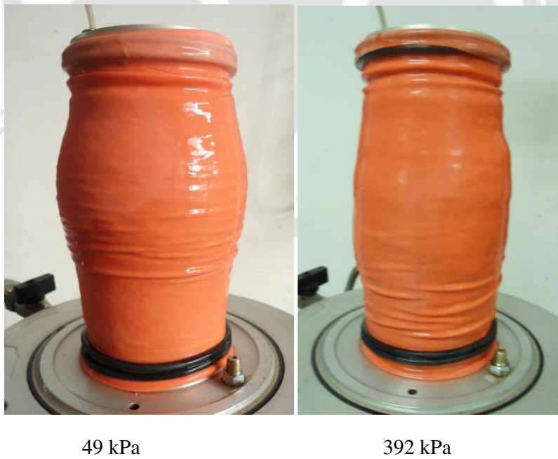
Fig.5.47 Failure mode of fiber reinforced loose soil ( D_r = 30\% , L = 20\text{ mm} , f_c = 2\% ): Influence of confinement pressure.
