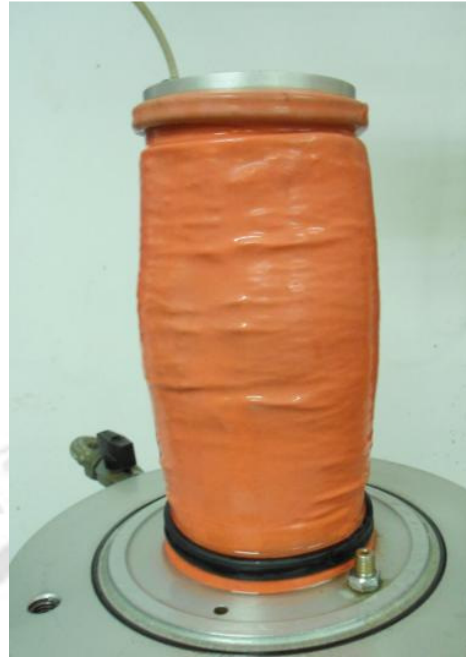
Fig. 4.7 Typical failure mode of geocell reinforced soil specimen ( D_r = 80\% , Geocell made of GT_1 , \sigma_3 = 196 kPa)
