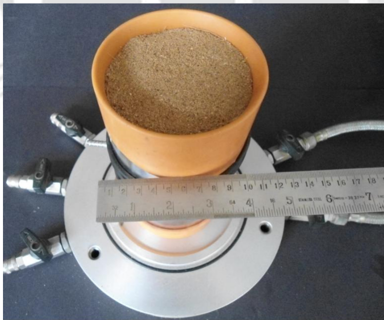
Fig. 3.10 Typical unreinforced soil specimen
