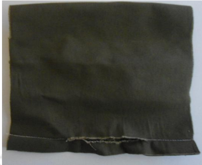
Fig. 4.9 Rupture of seam of geocell after test (Geocell made of GT 1 )
