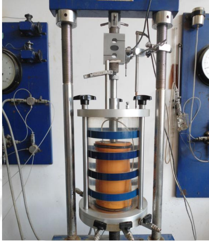
Fig.3.14 View of the test specimen placed in the triaxial compression cell.
