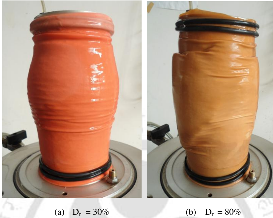
Fig. 5.30 Failure mode of fiber reinforced soil, lightly reinforced ( L = 20 mm, f_c = 2\% , \sigma_3 = 49 kPa): Influence of relative density of soil
