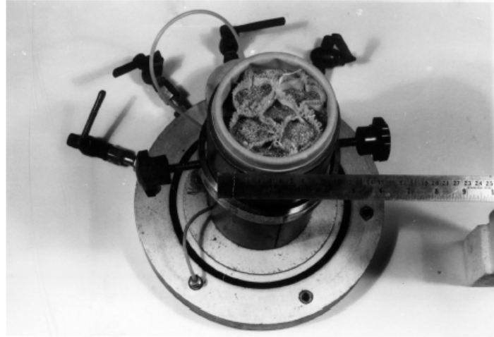
Fig 2.8 Typical test specimen with multiple geocells (Rajagopal et al. 1999)
