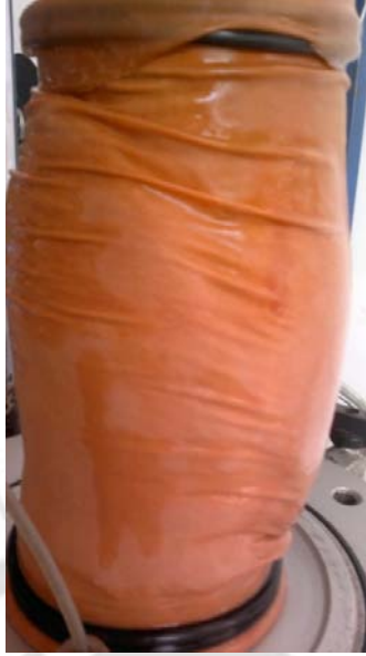
Fig. 5.3 Typical failure mode of fiber reinforced soil ( D_r = 80\% , L = 40\text{mm} , f_c = 4\% , \sigma_3 = 196 \text{ kPa} )
