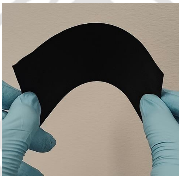
Figure 2.1. Photograph of a piece of the exfoliated reduced graphene oxide (rGO) sheet utilized as electrode in this research.
