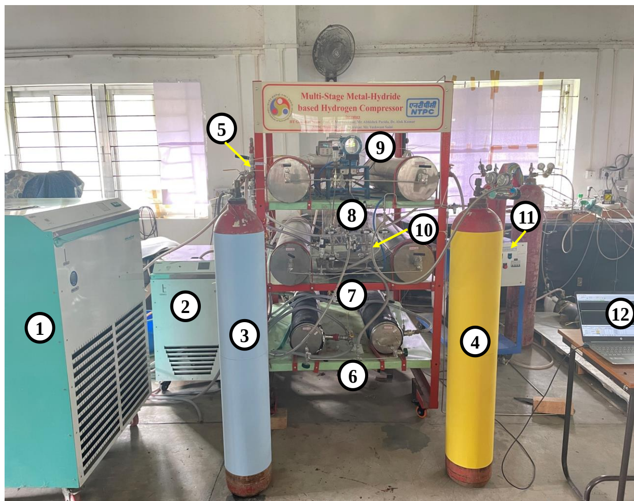
1-Cold recirculating bath 2-Hot recirculating bath 3-H 2 empty cylinder 4-H 2 supply cylinder 5- HTF circuit panel 6-First stage reactors 7-Second stage reactors 8-Third stage reactors 9-Coriolis mass flow meter 10-Gas circuit panel 11-Vacuum pump 12-PC
