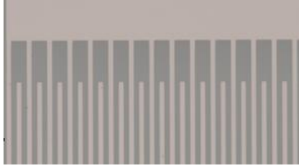
Figure 5.2 Optical microscope picture of the IDT pattern on the chrome mask plate.
