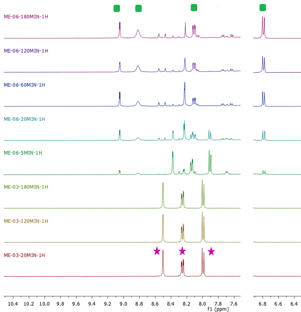
Figure 4.3.6.6: Stacked 1 H NMR diagram for (compound 2a + DIPEA (after 3 h, BnNH 2 added))
