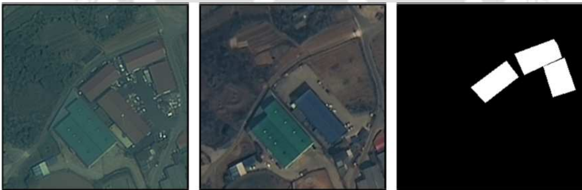
Figure 2.2: Visualization of CD task. Here, the white color is the actual change detected by the model depicted in the right image, and the left and middle images are the inputs.
