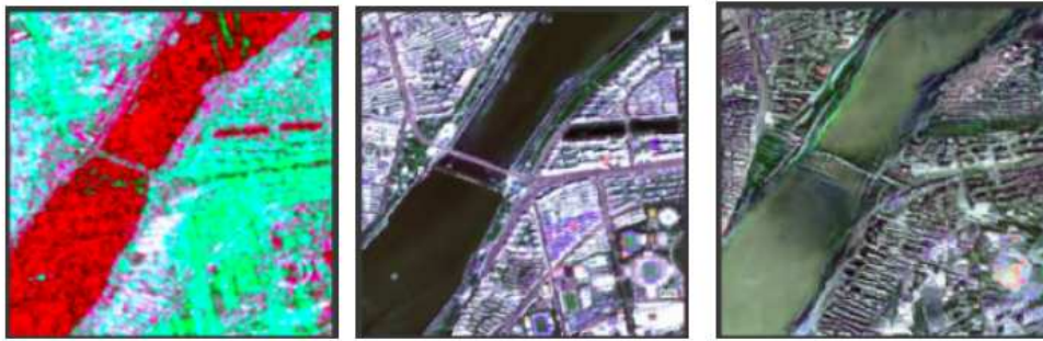
Figure 2.3: Visualization of SAR to Optical IT task. Here, left image is SAR input, middle image is sentinel 2 output, and right image is predicted output.
