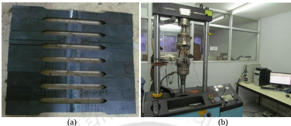
Figure 4.12 Image of the (a) Tensile samples (b) Instron 3382 universal testing machine
