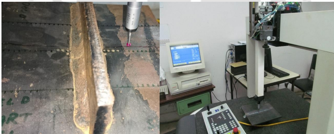
Figure 4.11 Measurement of angular deformation using CMM
