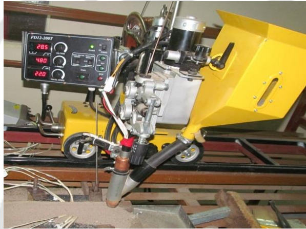
Figure 4.1 Submerged arc welding set-up
