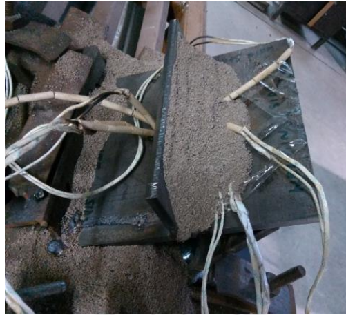
Figure 5.26 Welded sample with flux and thermocouples attached
