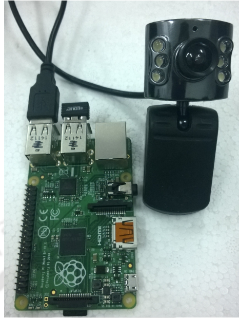
Figure 2.4: The Pi based Tartarus host interfaced to the Webcam
