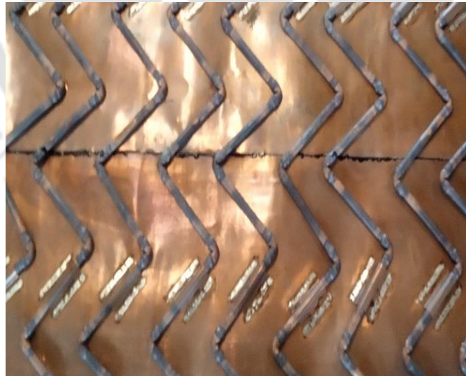
Fig. 3.7 Photograph of the collector with copper tubes
