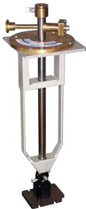
Figure 2.7: High temperature oven attached with VSM.
