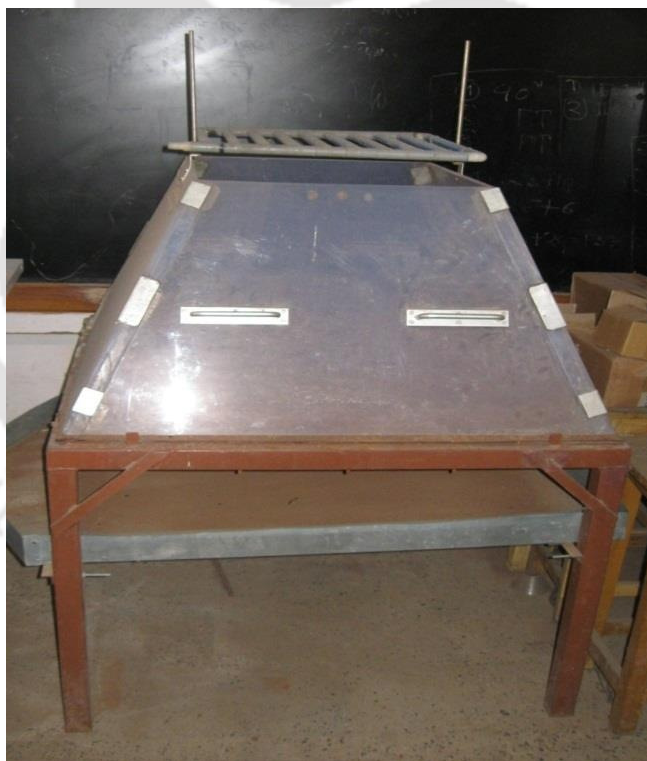
Fig. 3.8 Photograph of heap shaped column leach apparatus
