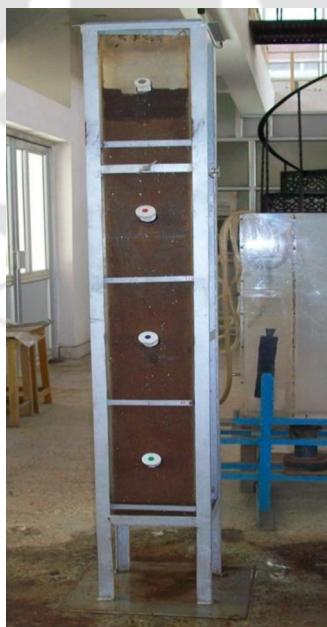
Fig. 3.4 Photograph of long rectangular column leach apparatus
