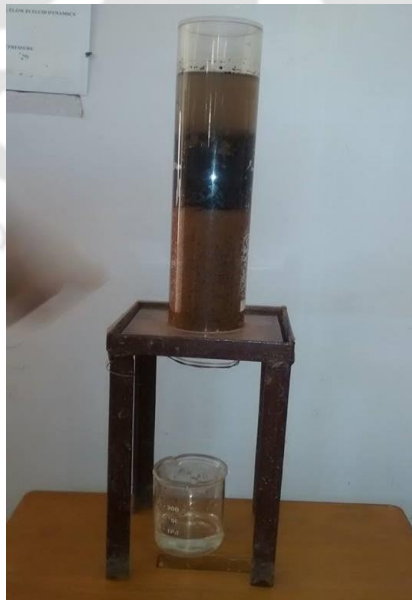
Fig. 3.6 Photograph of cylindrical column leach apparatus
