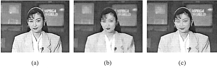
Figure 2.10: (a) Original image; (b) result of open-close (c) result of open-close by reconstruction.
