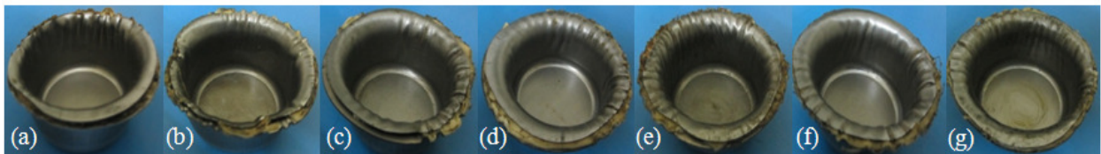
Fig. 7.19 Wrinkling behaviour of adhesive bonded sheets with different numbers of Cu wire reinforcements
