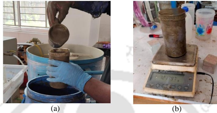
Figure 5-2: Measurement of fresh density (a) collection of pre-formed concrete mix in standard container, (b) weigh measurement of the container
