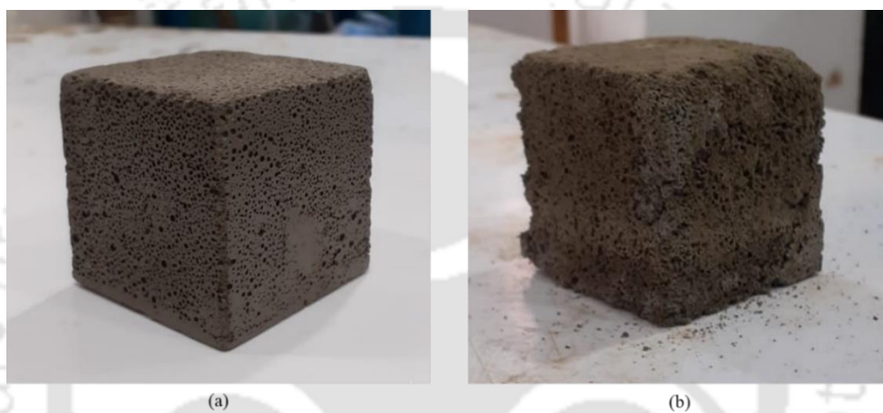
Figure 4-18: Images of demoulded specimen (a) Specimen with intact shape and edges (b) Specimen with distorted edges and shape
