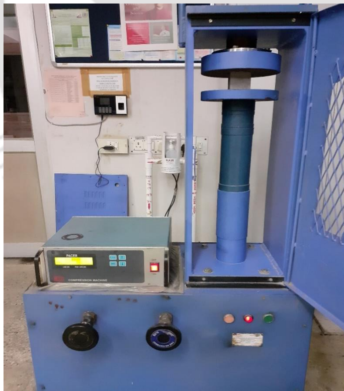
Figure 5-4: Compressive strength testing machine with a maximum capacity of 50KN
