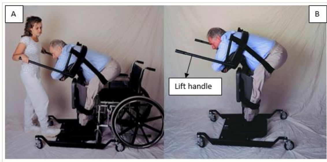
Figure 2-8 The Easy Pivot Mechanism, during lifting(A) and lifted up phase (B)
