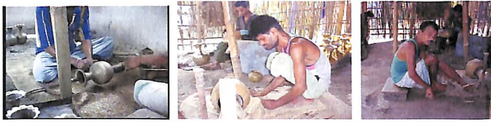
Fig. 20 Polishing through rope operated wooden shaft rotation.
