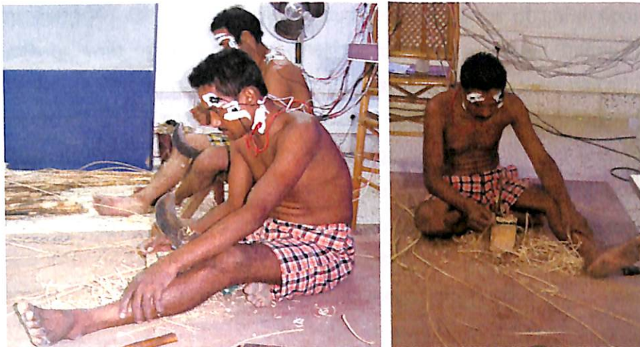
Fig. 35 While working with modified fiber making tool postural benefits are being evaluated with EMG
