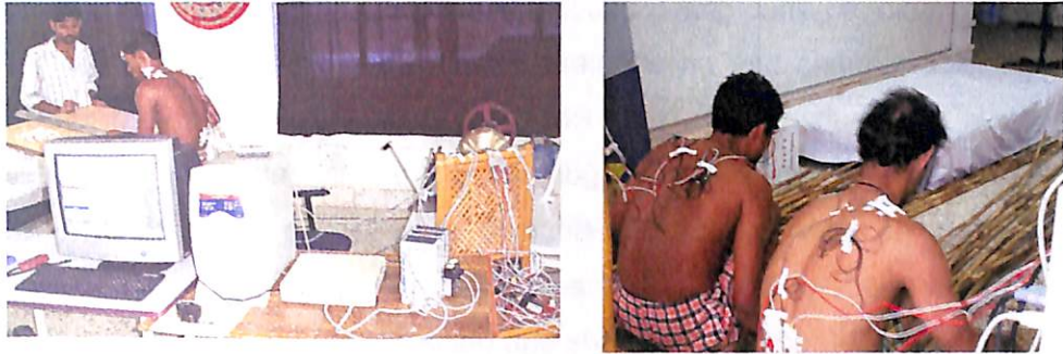
Fig. 30 Set up for recordings of EMG during performance of different cane crafts and brass metal activity
