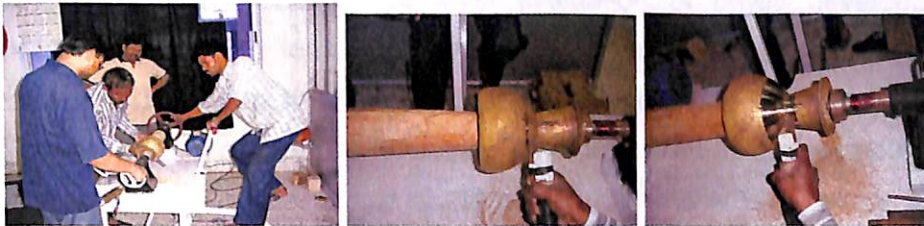
Fig. 47 polishing operation through shaft rotation and cutting tool, one is paddling and other one is engaged in polishing.
