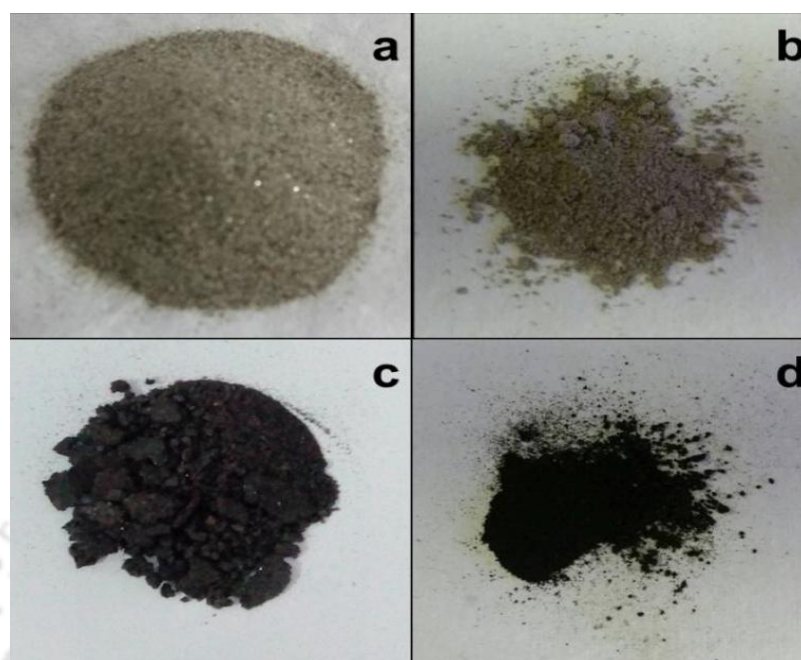
Figure 3.2. (a) Photograph of sand before and (b) after ball milling, (c) Photograph of sand–Fe–Cu nanocomposites prepared before and (d) after ball milling of sand.
