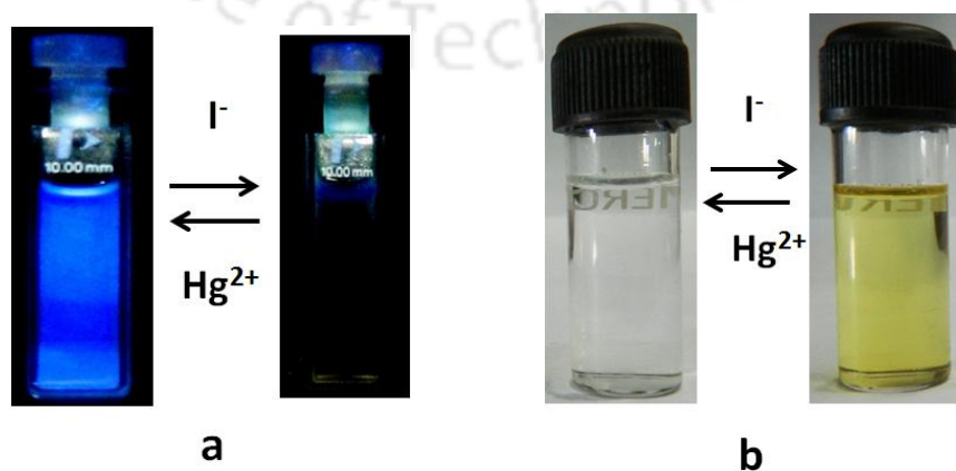
Figure 2.1 Color of the PPT solution in 4:1 THF/water under (a) UV light (b) naked-eye.
