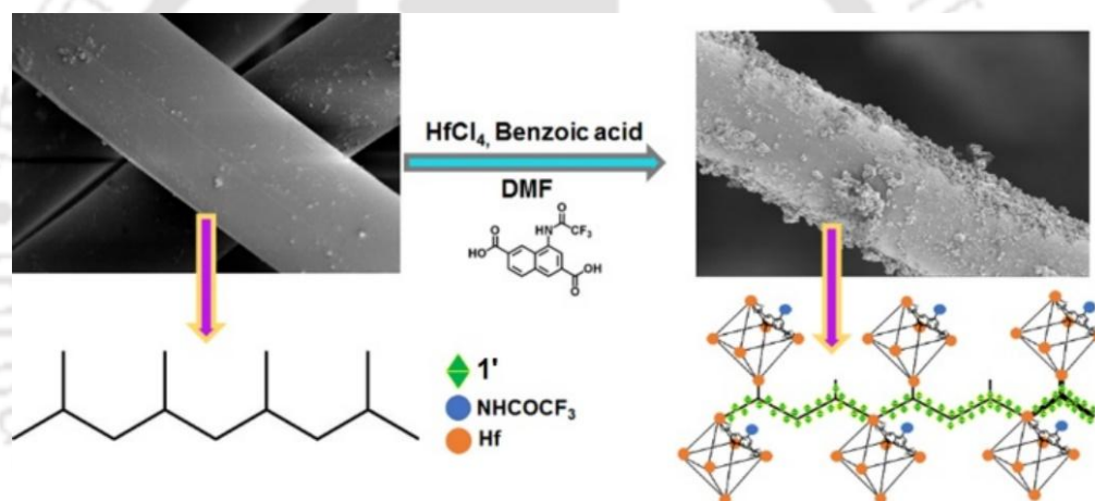
Scheme 2.1. Scheme for the single-step in-situ synthesis of 1'@PP in a solvothermal process.
