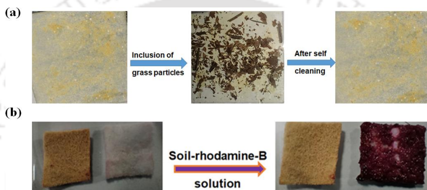
Figure 6 (a) Digital images of 1'@PP coated glass slide displaying self-cleaning nature. (b) Digital images of 1'@PP composite and PP-fabric before and after antifouling experiment.
