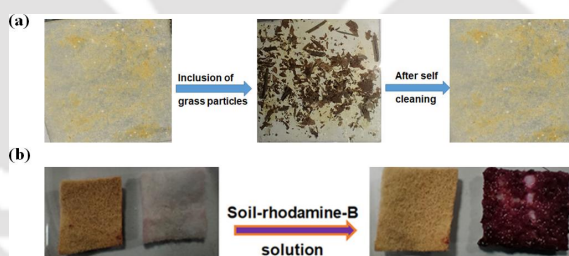
Figure 2.40 Digital image of 1'@PP coated glass slide displaying self-cleaning nature and (b) digital images of 1'@PP composite and PP-fabric before and after antifouling experiment.
