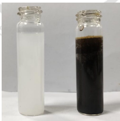
Figure 4.39 Change in colour of 3 + \text{Pb}(\text{CH}_3\text{COO})_2 aqueous mixture after the addition of hydrazine.
