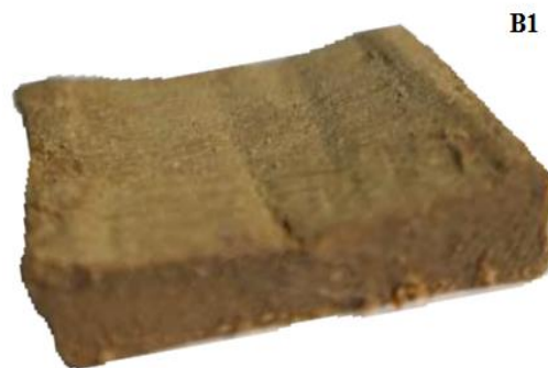
Fig. 4.3b Cross-sectional view of a clod specimen of DVM technique
