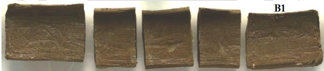
Fig. 4.3a Bentonite specimen in DVM technique during shrinkage process
