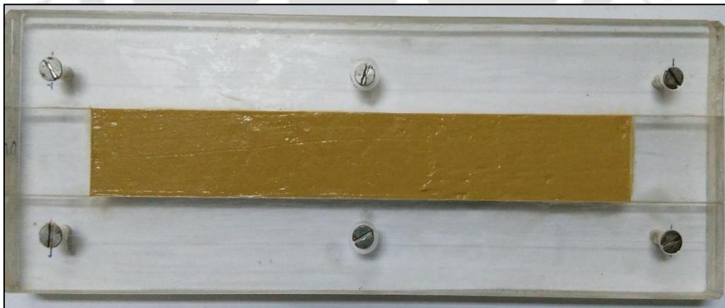
Fig. 3.8 Shrinkage box (200 x 30 x 10 mm) with specimen at the initial state
