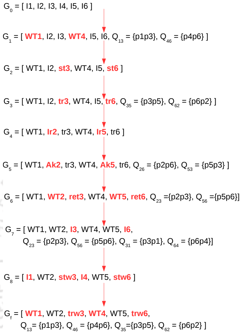
Figure 4.10: Global State Transitions of CFSMs in Fig. 4.9
