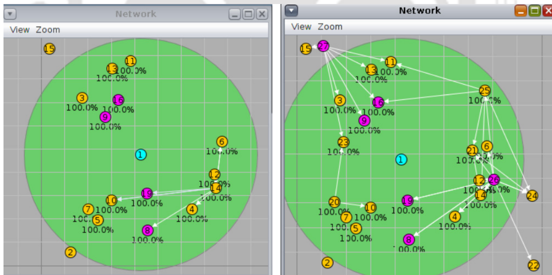
Figure 5.7: Snapshot of 4, 6 malicious nodes during mixed rate DDoS attack
