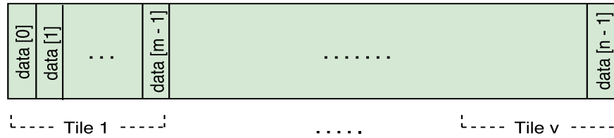
Figure 6.16: Tiled Data layout for parallel processing.
