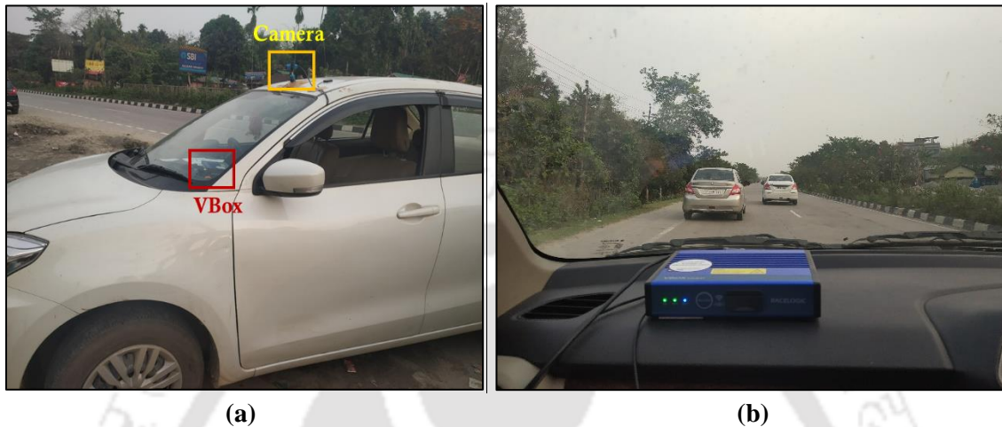
Figure 3.10. A depiction of the instrumented vehicle and video VBox placed in the dashboard of the following car
