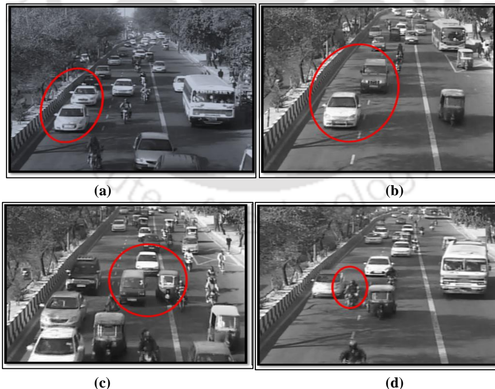
Note: CS: centerline separation; LG: Longitudinal gap; LF: Left-front; RF: right-front; r_x : pore size Figure 2.2. Following behaviours in disorderly traffic (a) Car-following (b) Staggered-following (c) Two-leaders following and (d) Filtering
