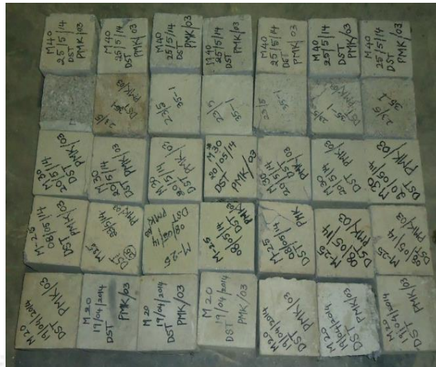
Fig.3. 4 Cube samples of five mix designs (M 20–M 40) after the compression test
