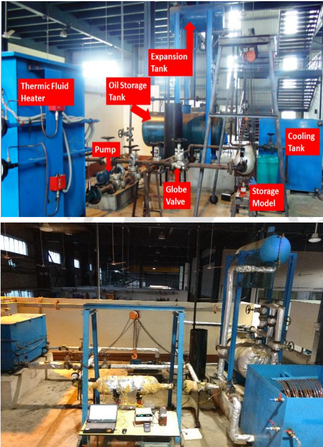
Fig.4 2 Experimental set-up to study the SHS prototypes (a) before insulation (b) after insulation.
