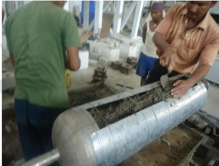
Fig.3. 6 Arrangement of the concrete fill inside the M2 storage prototype on the Vibrator
