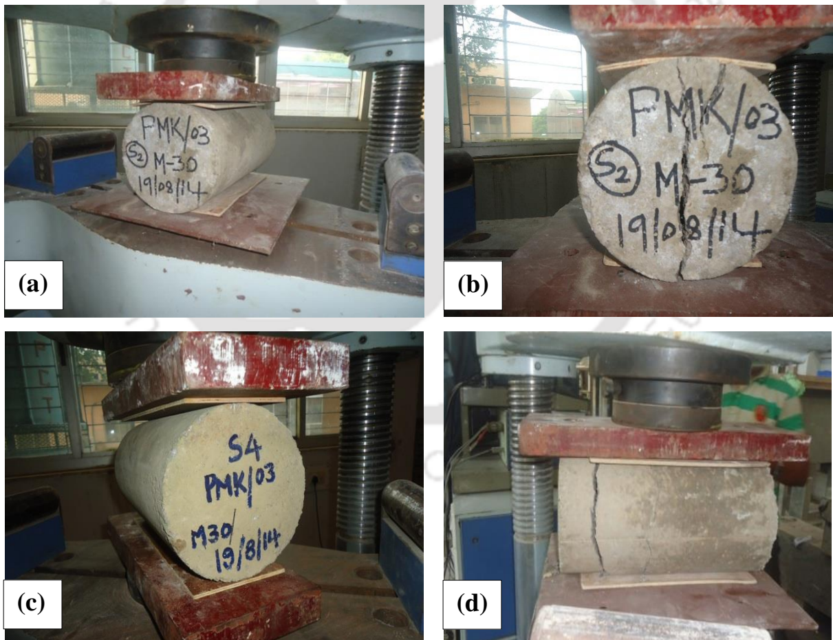
Fig.3. 5 Specimens before and after split tensile test (a & b) 7 days (c & d) 28 days
