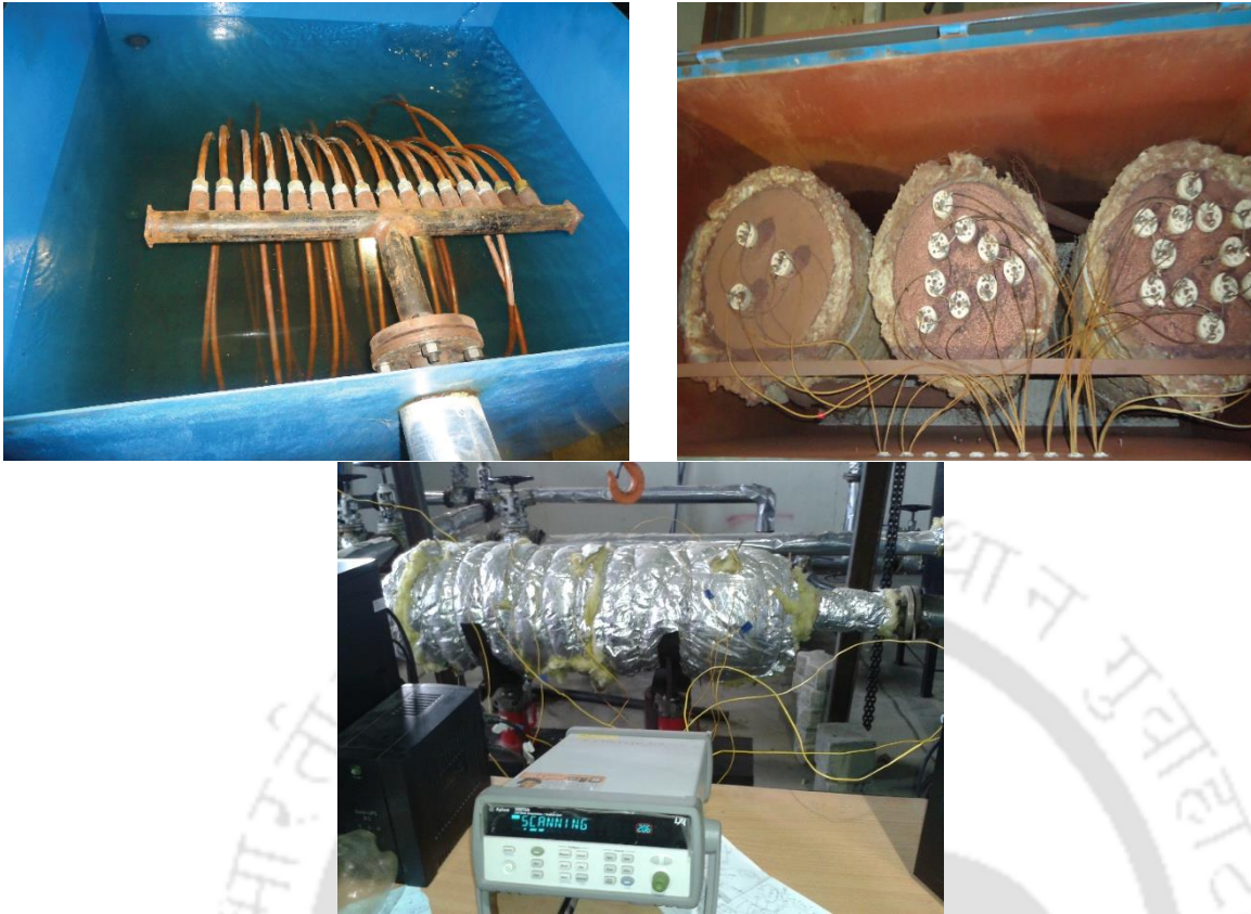
Fig.4 3 Experimental setup (a) water based coil-type heat exchanger, (b) the heating chambers and arrangement of the heaters and (c) model connected with thermocouple and data acquisition system.
