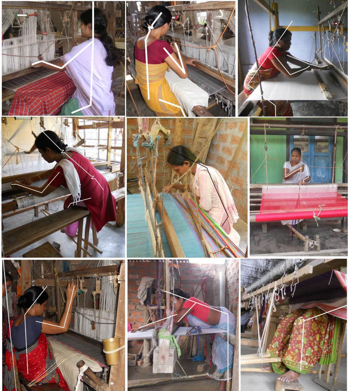
Figure. 2.19 Stick diagram of REBA posture analysis of individual body parts
