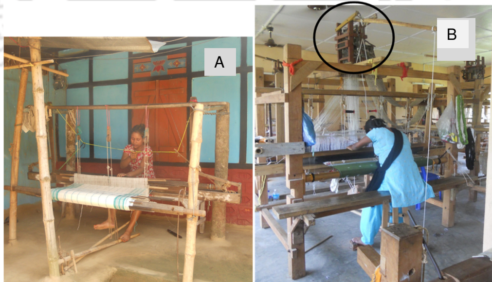
Figure 2.15 Picture showing (A) Domestic loom without Jacquard (B) Commercial loom with Jacquard
