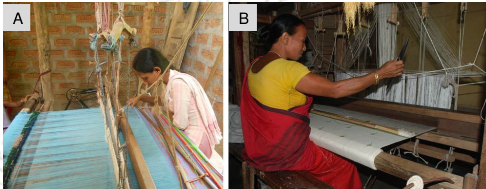
Figure.2.-18 Motif formation in (A) Domestic loom and (B) Jacquard loom
