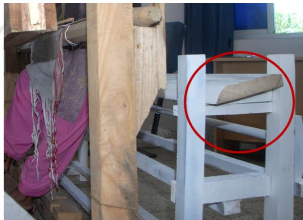
Figure. 3.18. Inclination of plank showing 5° angle
