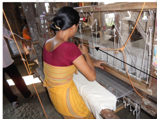
Figure. 3.3. Picking operation with flying shuttle
