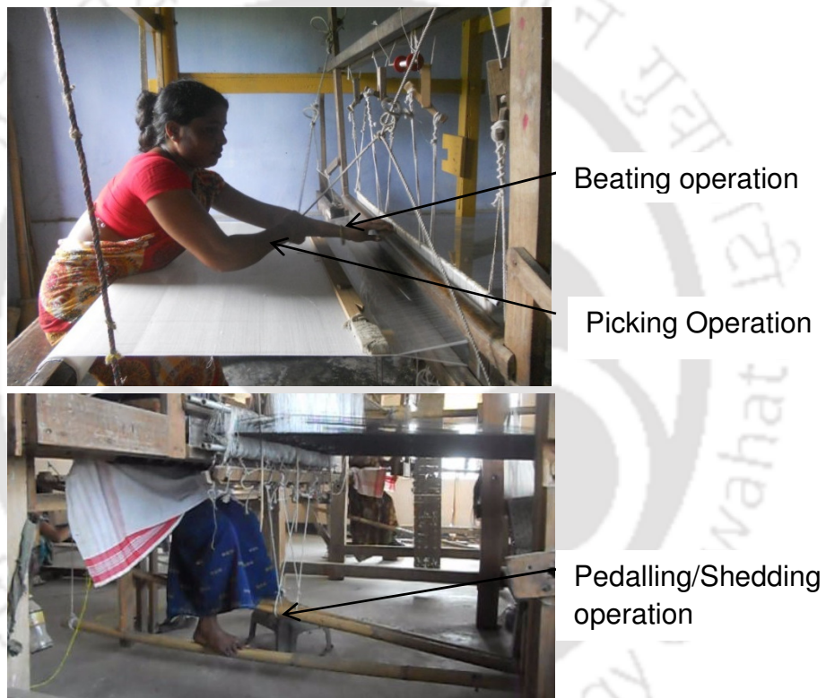
Figure. 2.13. Body segments involved in weaving subtask: Right hand for picking, Left hand for beating, Right Leg for pedalling or shedding
