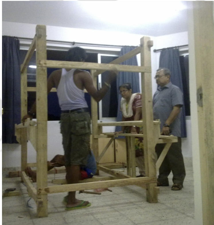
Figure.3.6. Simulated loom in control laboratory environment to undergo ergonomic design modification by participatory approach
