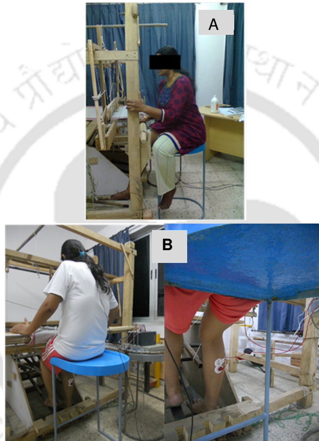
Figure 3.43 EMG recording with (A) Existing and (B) Modified Pedal on single seat
