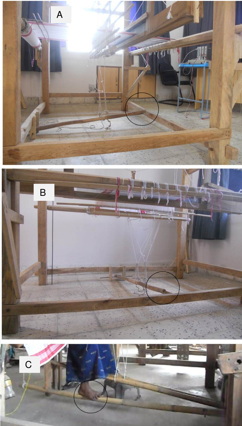
Figure.3.22. Existing pedal of the present handloom (A) Side view (B) Front View and (C) Mode of operation with Right Leg
