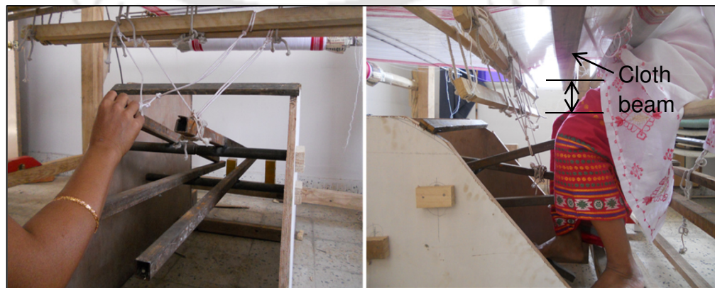
Figure. 3.26. Trial pedal prototype showing increased height of the pedal from floor
