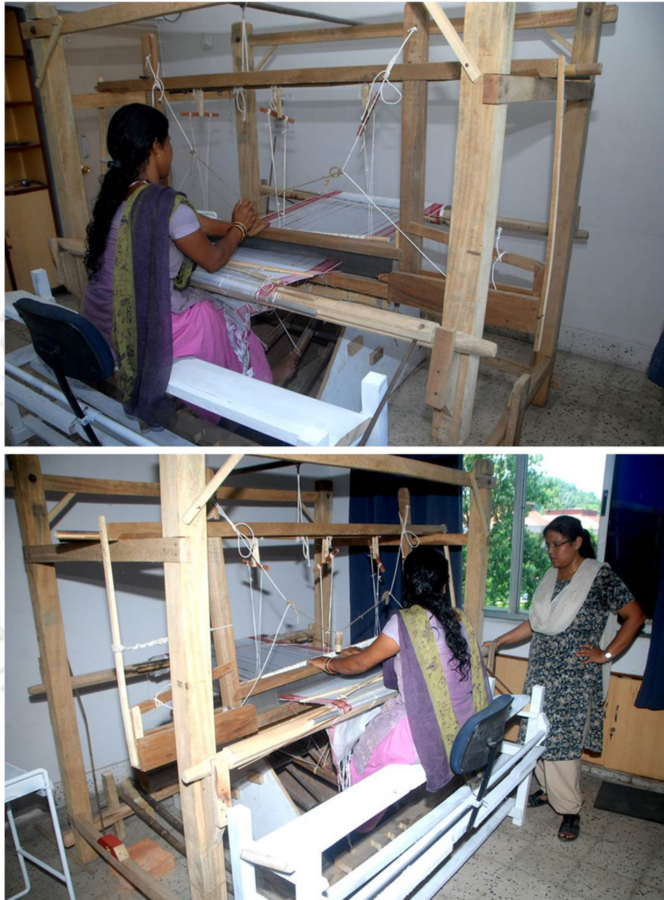
Figure. 3.45. Final plank design with adjustable height and movable backrest
