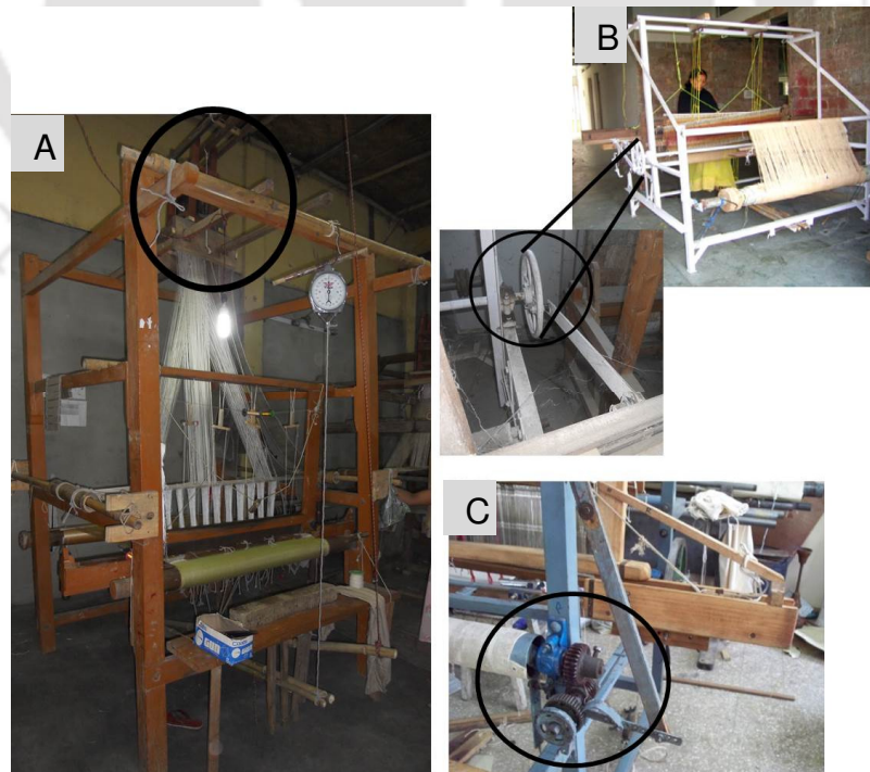
Figure. 3.4. Technological Up-gradation in the handloom industry, (A) Jacquard for motif (B) Crank for beating motion (C) Gear for Take-up & let off motions.
