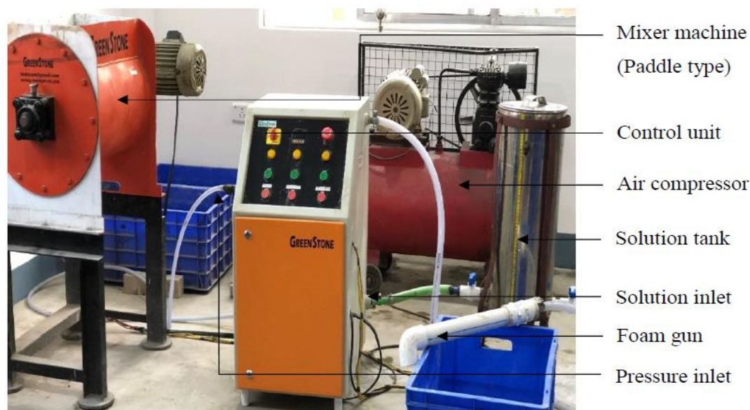
Figure 4-2 Foam generator set up
