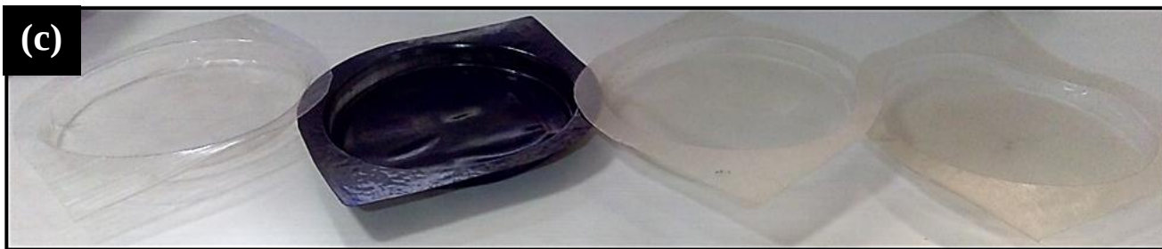
Figure 6.19: The predicted shelf-life for the (a) oil-based products (especially rapeseed oil) and (b) dairy based products using the PLA nanocellulose based composite films produced with the different compatibilizers. (c) Molded plates from reactively extruded PLA/CNC films for storage of food products with different compatibilizers (i) PLA/DCNC-S-1p, (ii) PLA/DCNC-S/Carbfiber, (iii) PLA/DCNC-S/Cellulose and (iv) PLA/DCNC-S/Olive Oil.
