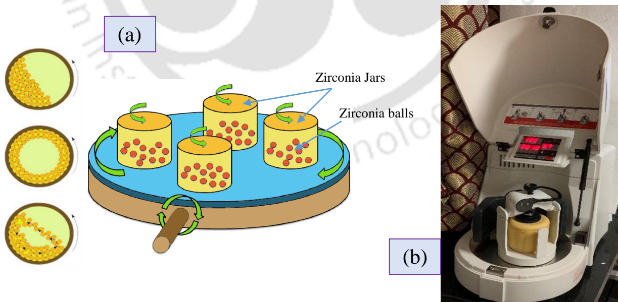
Figure 2.2: Schematic representation of how a planetary Ball-Mill works. Image on the left (a) shows the cascade action that happens inside the zirconia jar during the operation and the image on the right (b) shows the photograph of the Ball-Mill that was used in this work.
