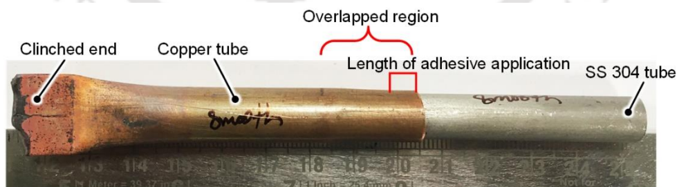
Fig. 7.3 Air leak test sample
