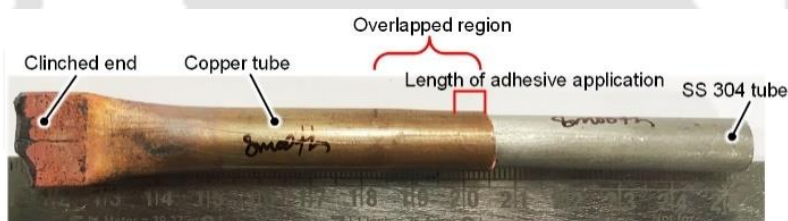
Fig. 6.15 Electromagnetically assisted adhesive Cu-SS joint sample at 3.4 kJ of discharge energy for leak test
