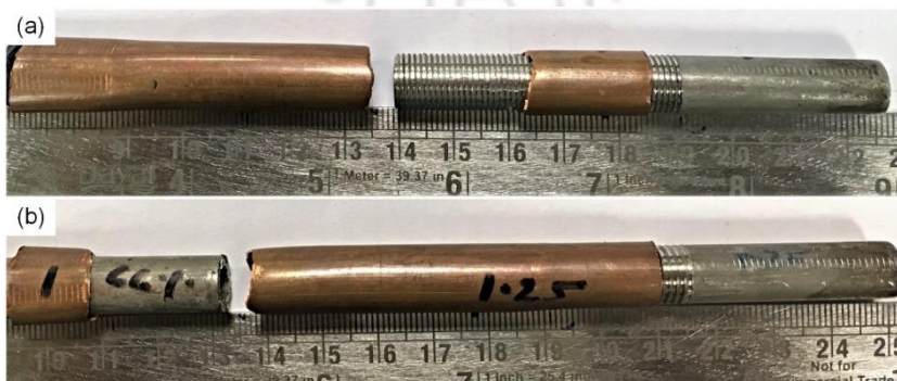
Fig. 5.19 Crack failure mode obtained for samples at 4.4 kJ of discharge energy for the pitch of (a) 1 mm and (b) 1.25 mm
