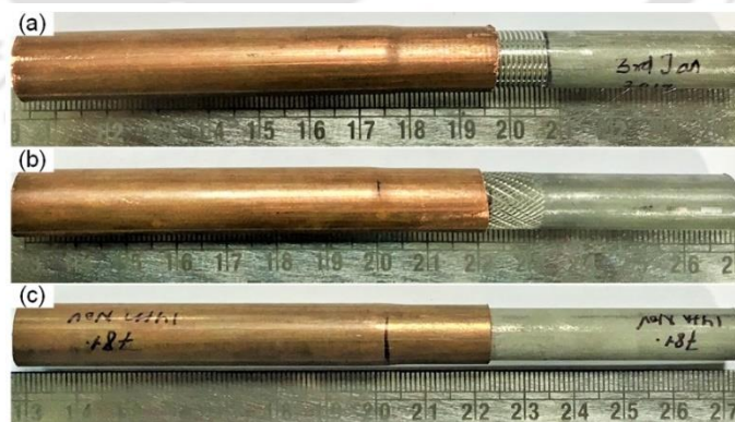
Fig. 3.8 Crimped samples for three different surface profiles prepared at 6.2 kJ of different discharge energy levels
