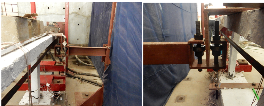
Figure 6.3 Lateral restraint setup to prevent out of plane movement of RC frames during testing
