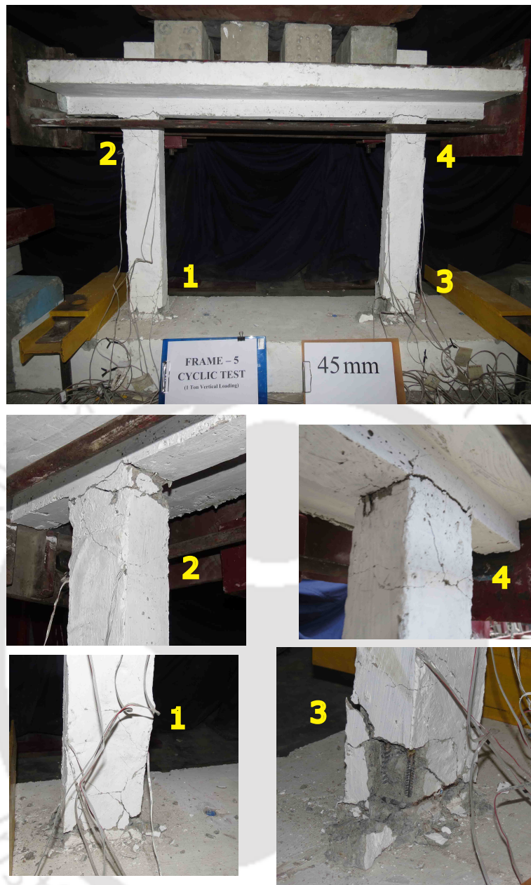
Figure 6.13 Damaged frame-A2 due to main shock damage corresponding to 45 mm displacement by slow-cyclic testing (10 kN gravity loading)
