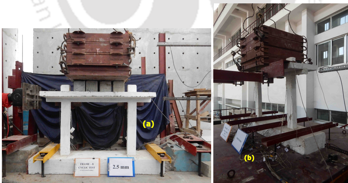
Figure 6.2 Experimental setup shown for (a) slow-cyclic, pseudo-static tests and (b) dynamic tests
