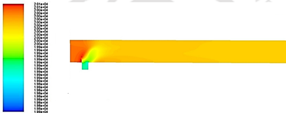
Fig. B.4(a) Pressure contour of T-junction design gas mixer with nozzle inclined at an angle of 90^\circ
