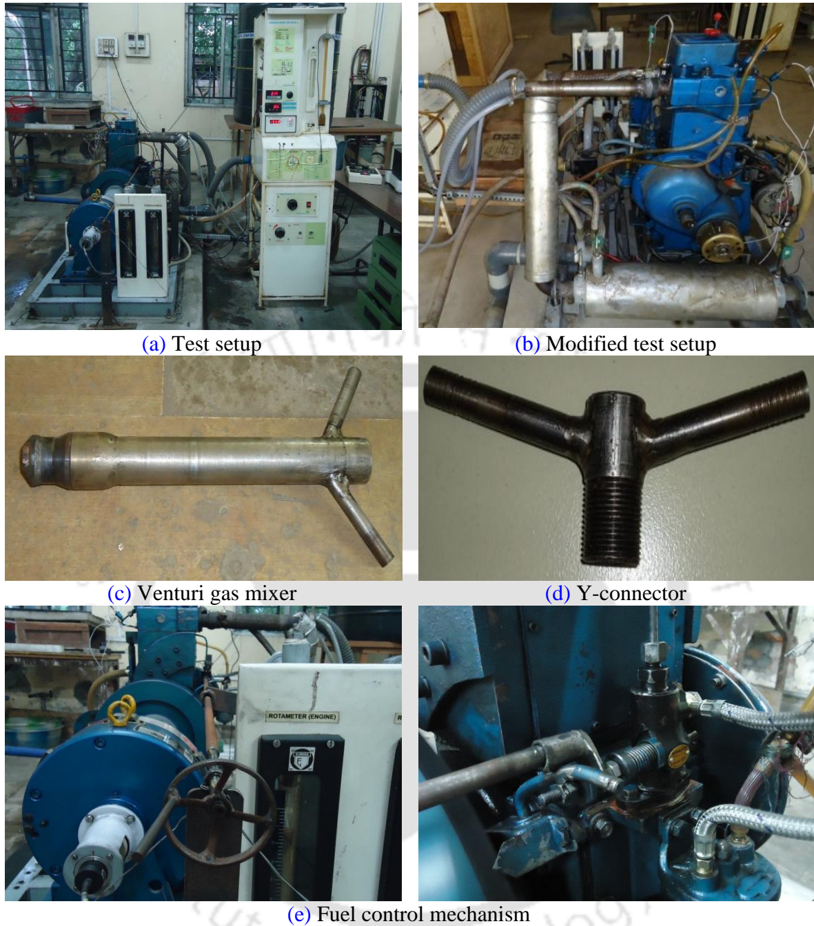
Fig. 3.3 Experimental facility and key components
