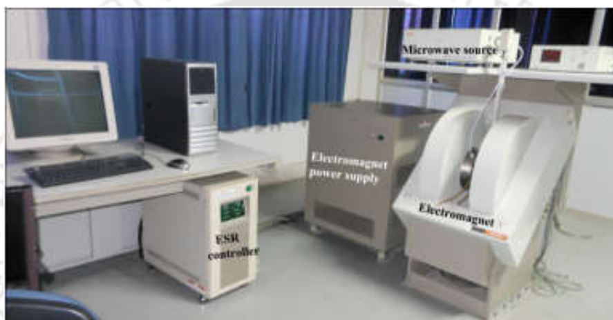
Figure 2.13: Photographic view of ESR spectrometer (JEOL, JES-FA200).
