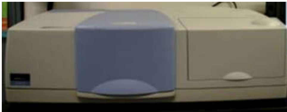
Figure 2.8: Photograph of the Diffuse Reflectance Spectrometer (Perkin Elmer, LAMBDA 750)
