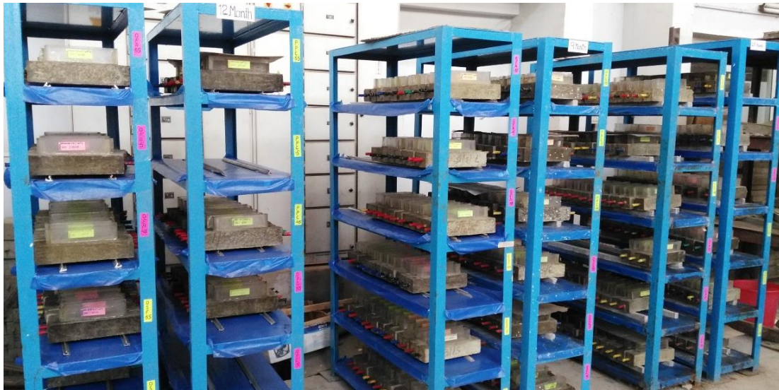
Prismatic specimens in the laboratory subjected to wetting-drying
