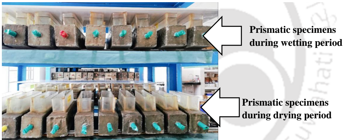
Prismatic specimens in the laboratory subjected to wetting-drying
