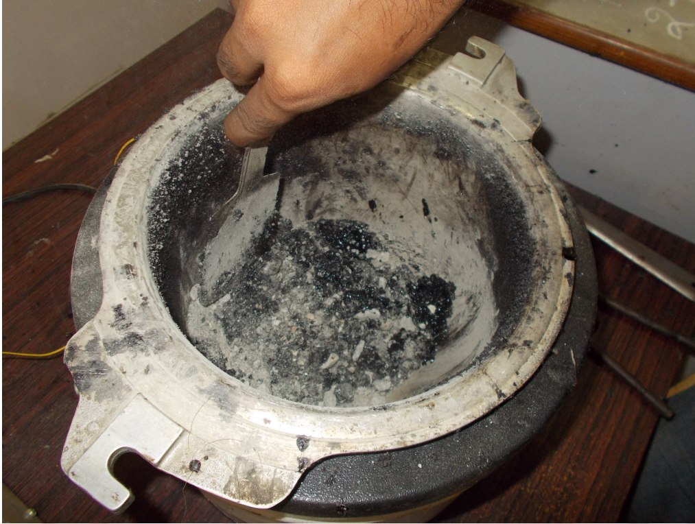
Figure 3.9: Mixing of batched aggregates and bitumen
