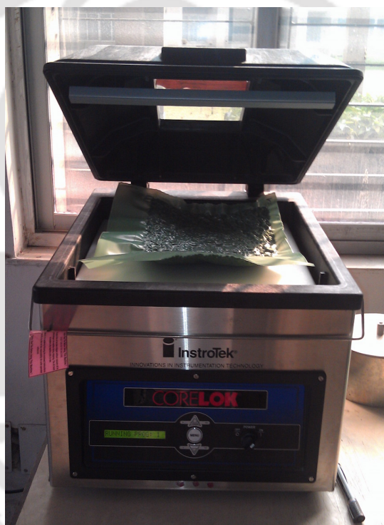
Figure 3.11: Determination of G_{mm} for loose mixes using Corelok™ instrument
