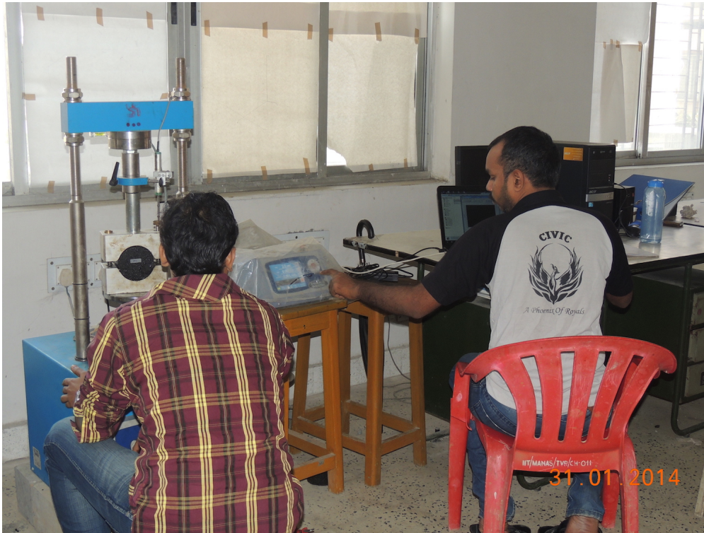
Figure 3.12: Testing of Marshall Samples for Marshall stability
