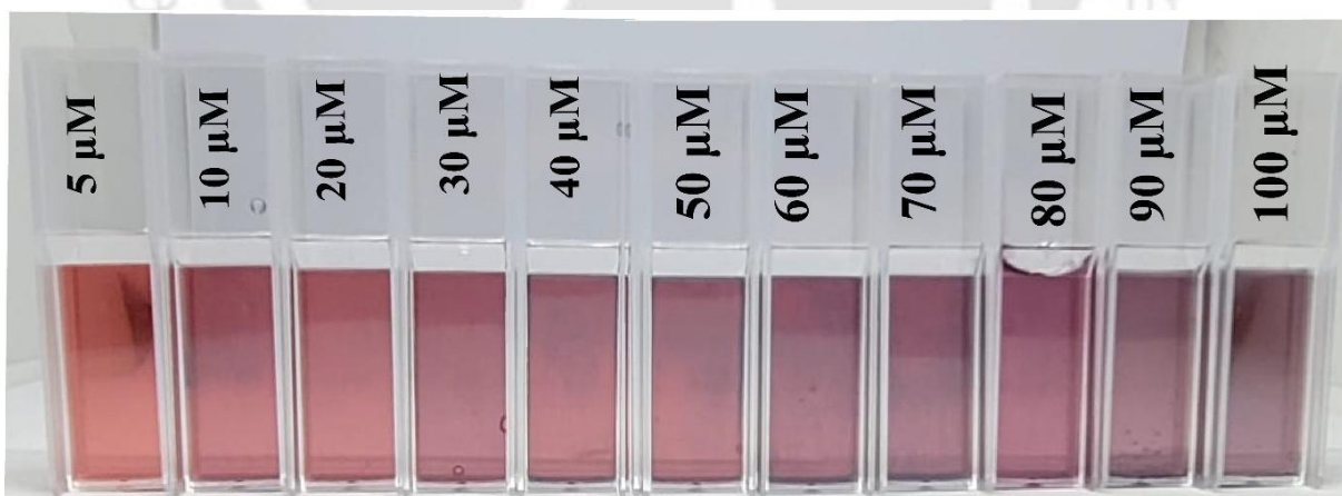
Figure 4.11: Colorimetric sensing response of AuNP-DSP system showing a progressive change in solution color with gradual increase in DSP concentration (5–100 \mu\text{M} )
