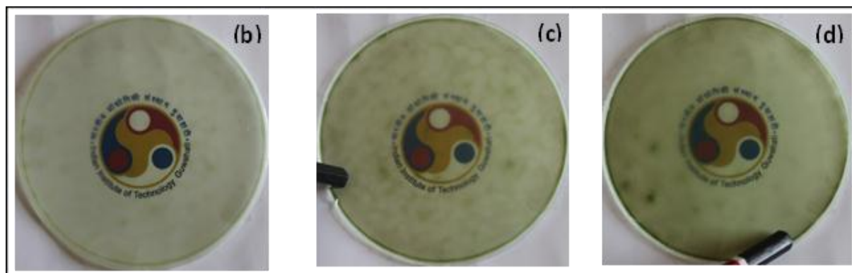
Figure 5.10 Transparency of neat PMMA, (i) PMMA/clay, (ii) PMMA/Co-Al LDH and (iii) PMMA/Ni-Al LDH nanocomposites with (b) 3, (c) 5 and (d) 7 wt.%
