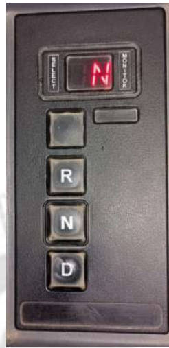
Figure 1.12: Gear mode control panel (Source: Author's field study, 2023).
