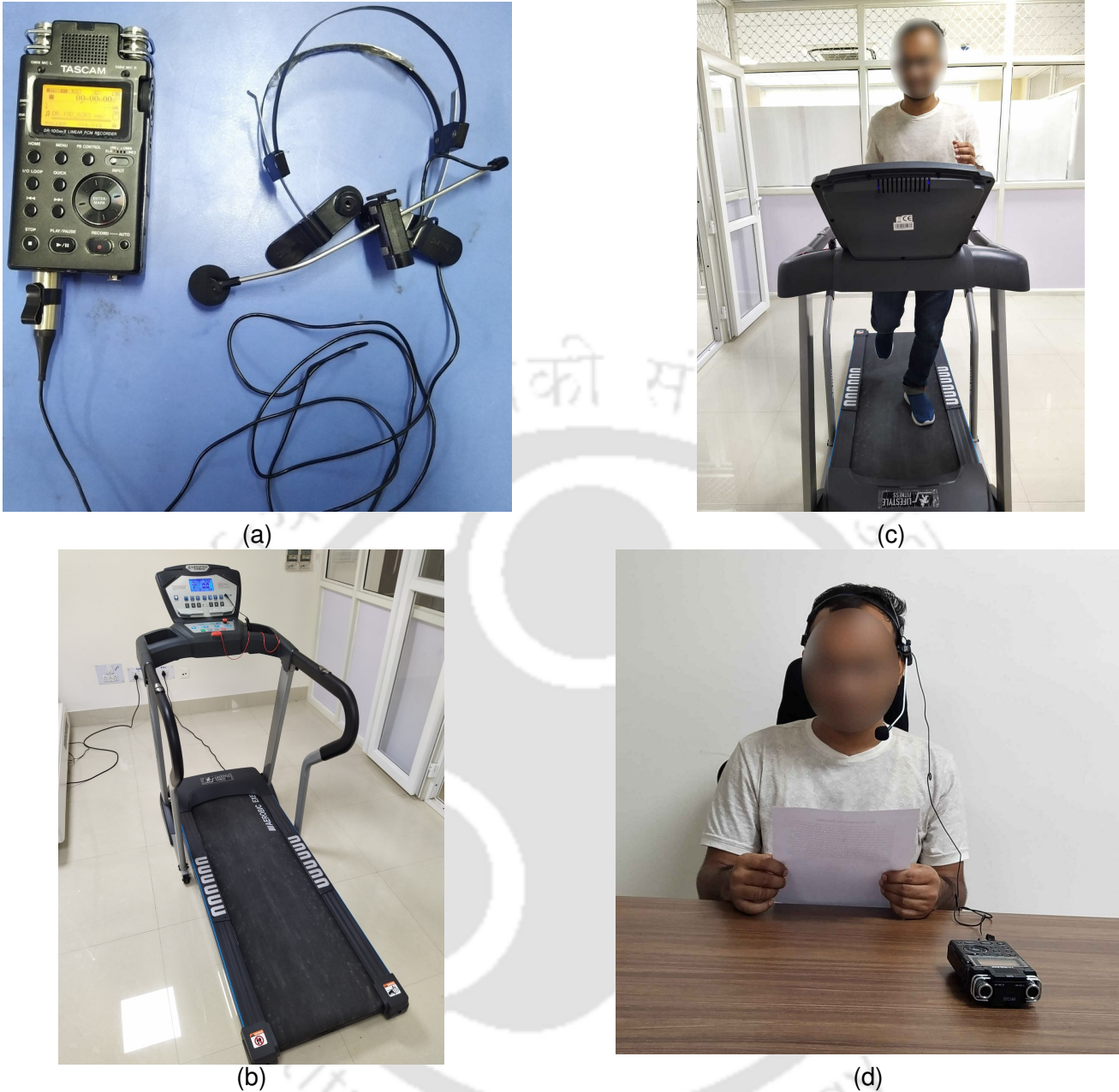
Figure 3.2: (a) and (b) show the instruments needed for recording (Tascam-DR-100MKII recorder, Shure head-worn microphone) and exercising (treadmill), (c) treadmill run exercise by a participating speaker, (d) representation of speech utterance recording at pre and post-exercise cases.
