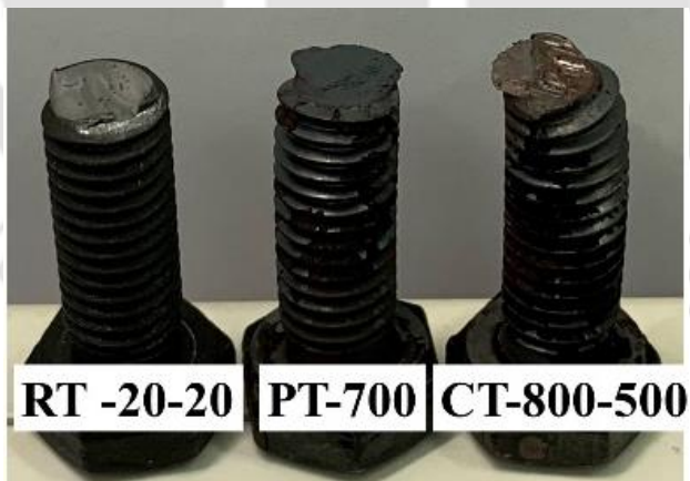
Figure 4-5 Typical tested specimens in shear tests
