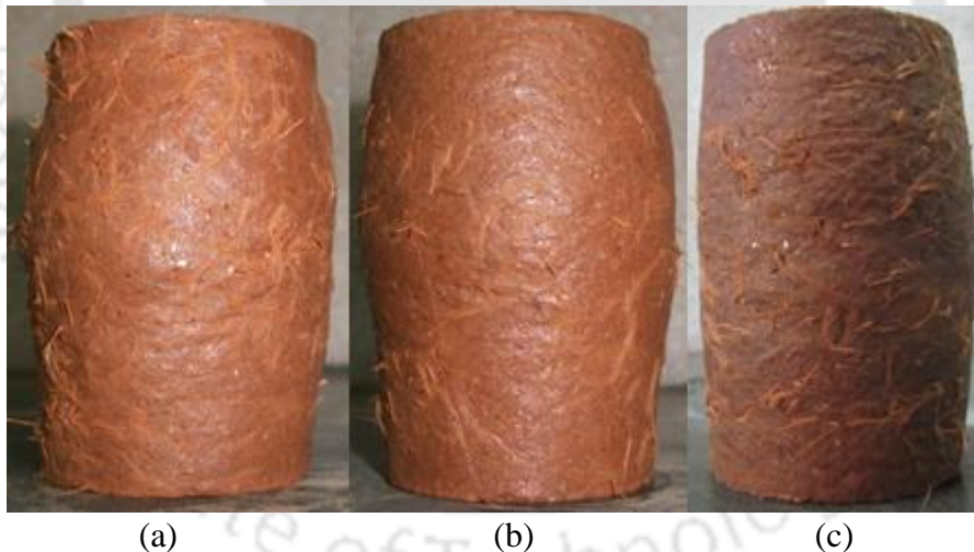
Fig. 6.6 Effect of confining pressure on deformation patterns of specimens reinforced with 0.75% fibres of 20 mm length and moulded at OMC and MDU (Series 1): (a) \sigma_3 = 100 kPa; (b) \sigma_3 = 200 kPa; (c) \sigma_3 = 400 kPa
