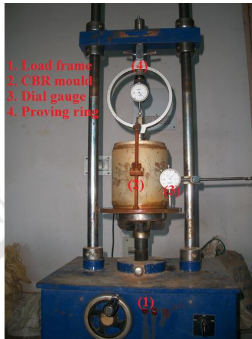
Fig. 3.5 Details of CBR testing equipment
