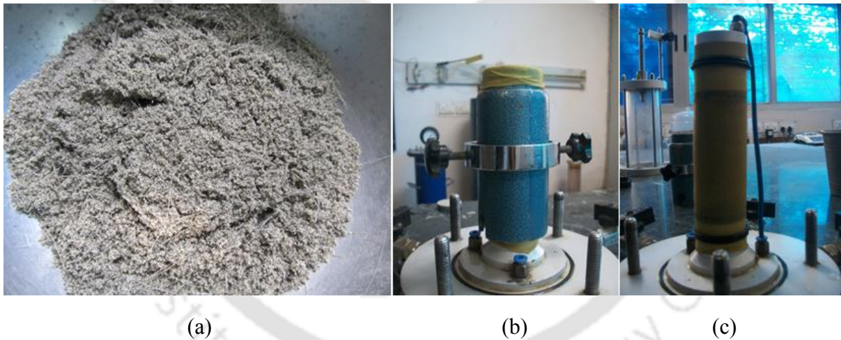
Fig. 3.8 Typical pictures of (a) sand-fibre homogeneous mix, (b) specimen preparation with split mould, and (c) test specimen
