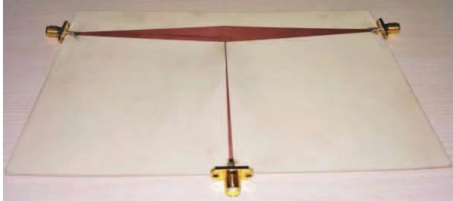
Figure 4.10: Photograph of the prototype fabricated T-junction power divider.
