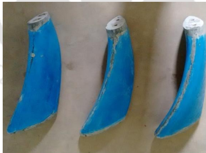
Figure 3.4: Fabricated helical fiberglass blades
