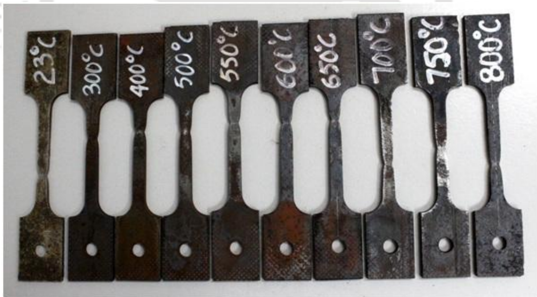
Figure 3.42: Typical failed specimens of 50 \times 50 \times 2.9 cross-section after tensile coupon tests under post-fire condition
