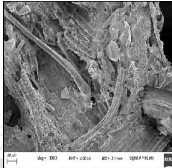
Fig. 6.48. After Electrohydrolysis Pre-treatment
